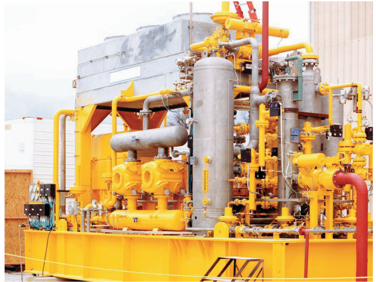
Model JGH/4, electric motor driven, for offshore Nigeria
